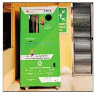
GREEN INITIATIVE: A reverse vending machine enables a person to insert a used plastic bottle (200 ml to 2.5 litres) or aluminium beverage can in exchange for a reward coupon
