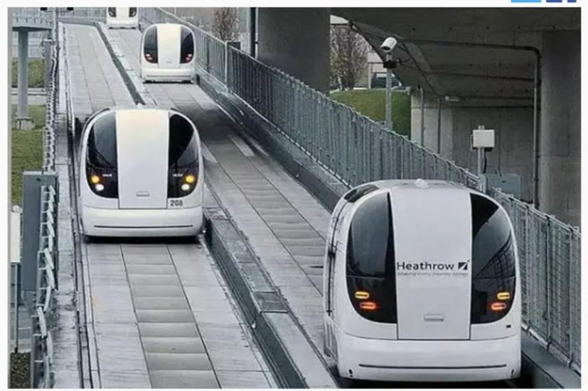
Driverless pod taxis are small automated vehicles operating on a network of specially built guideways.
