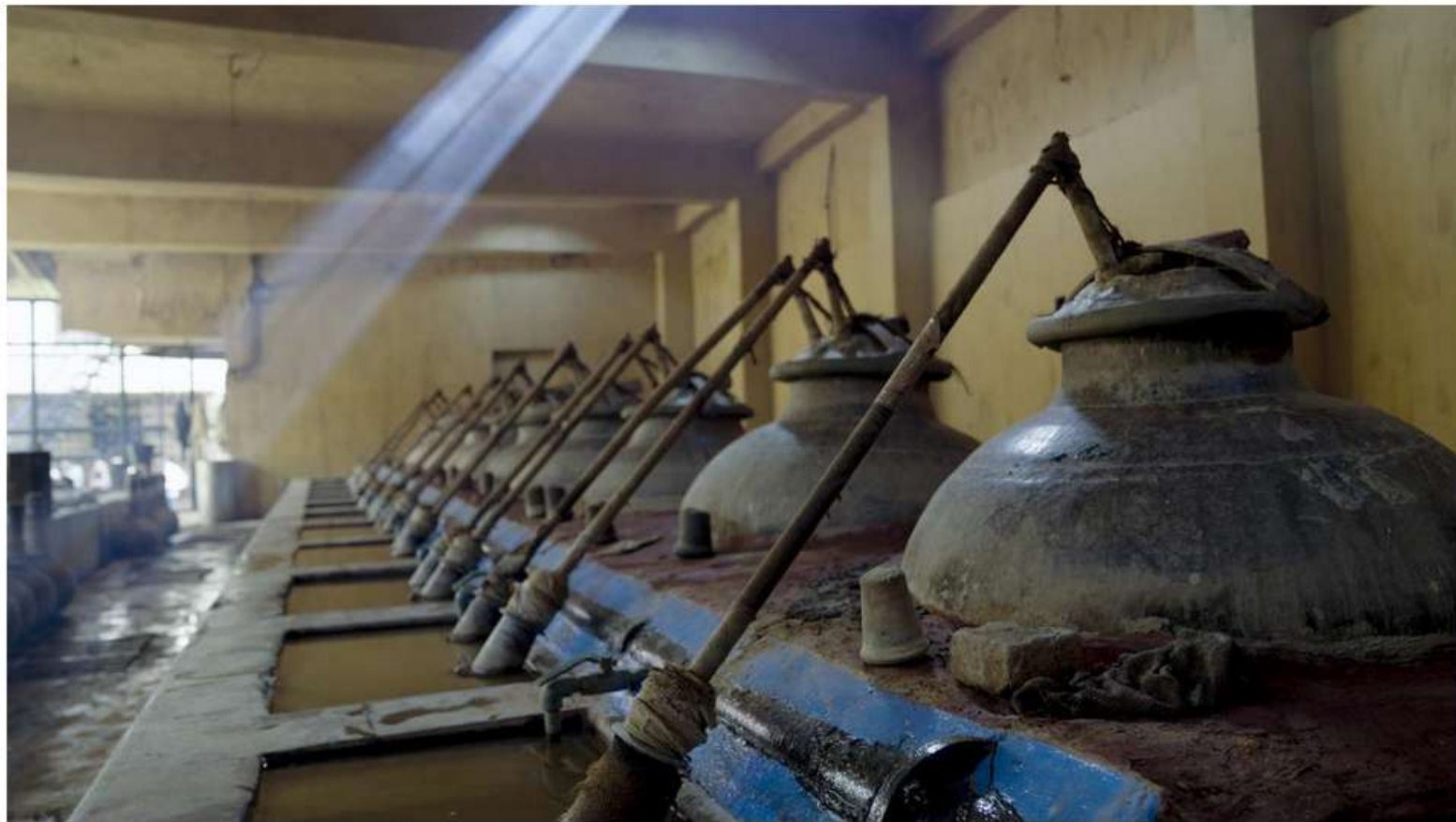
The traditional hydrodistillation equipment used in making attar. | Photo Credit: Richard Kujur
