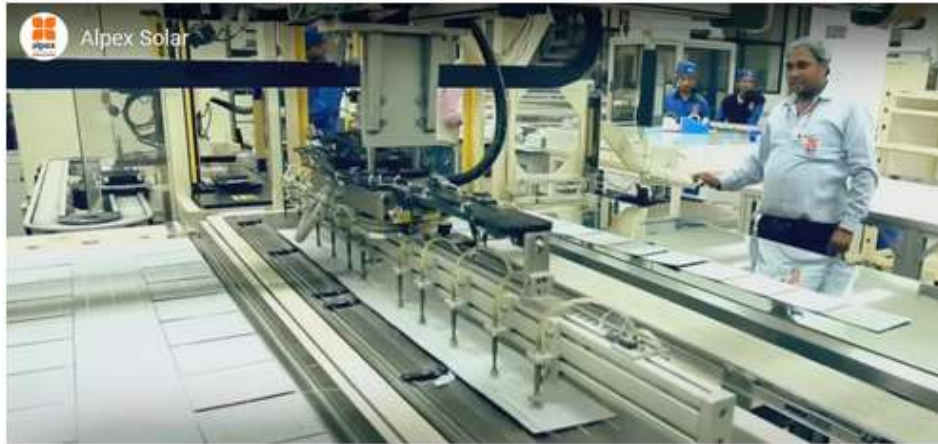
Tabbing and stringing at Alpex Solar production floor in Greater Noida Alpex Solar
