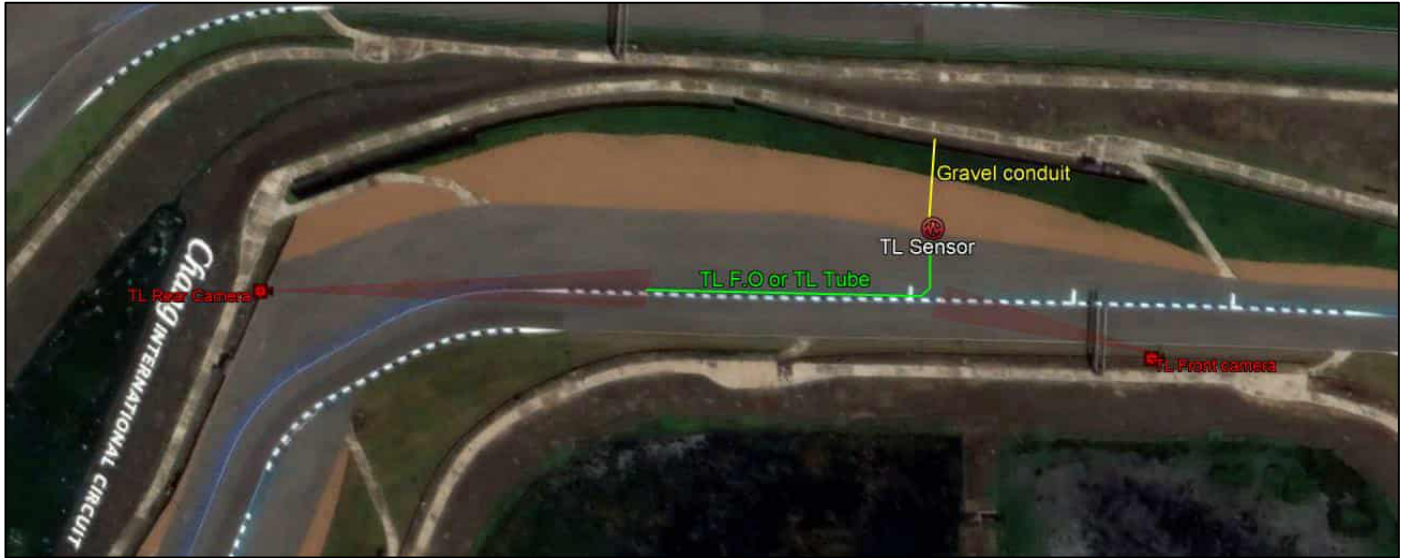
TRACK LIMITS DETECTION SYSTEM OVERVIEW
