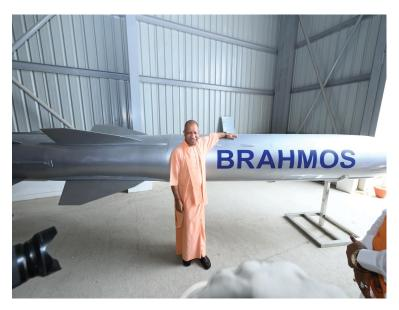
The BrahMos missile, developed through a joint venture between India's Defence Research and Development Organisation (DRDO) and Russia's NPO Mashinostroyeniya, is recognised as one of the world's fastest supersonic cruise missiles. It boasts a range of **290 to 400 km** and a top speed of **Mach 2.8**.
